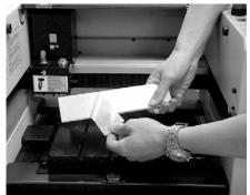
Step 2: Align each strip over the existing table and apply one section at a time.
