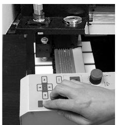
**Step 8**: Again, using the keypad, press the <u>Z</u> key to lower the spindle head so the bottom of the depth-nose gauge rests directly on top of the Corian<sup>®</sup> strip.
