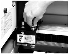
Step 6: Adjust the depth-nose gauge so the cutting tool is flush with the bottom of the gauge (or just slightly inside).
