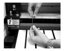
Step 5: Secure the cutting tool into the Spindle Unit.
