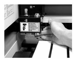
Step 14: (*This step is optional but can save time in the cleaning process*). Slip the vacuum-hose adapter around the depth-nose gauge and secure it by tightening the thumbscrew.
