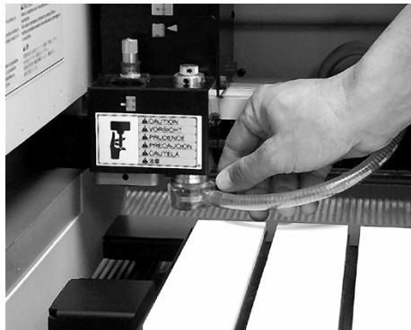
20. Set the spindle speed dial knob to the maximum setting.
