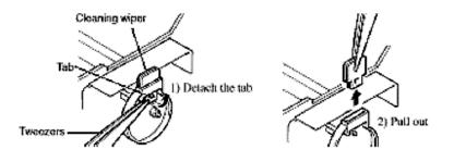
3. Use tweezers to attach the new cleaning wiper.
