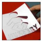
3. Weed away tactile material to reveal pictogram and text, ready for installation.
