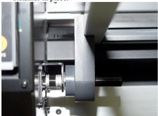
Step 3c - Ensure the Left Shaft Bracket fits snugly against the Left Media Retainer as shown.
