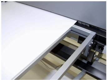
Step 10c - Move a support bar under the right edge of the sheet. Ensure the remaining bars are spaced underneath the sheet to prevent the media from bowing.
