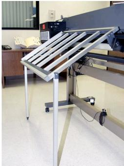
Step 4b - Attach the Rear Struts to Rear Table Top using medium screws.
