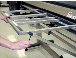
Step 8f - Place Front Table Top onto Printer Brackets or Printer Apron. Attach each strut to the Front Table Top with long screws.
