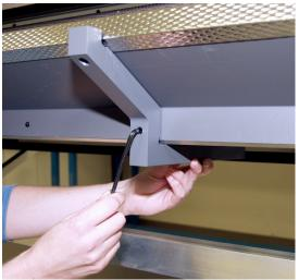
Step 7b - Lock down the Left Printer Bracket just enough to hold the bracket in place without the metal piece falling.
