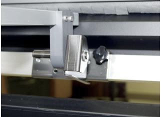
Step 3d - Attach the Right Roll Shaft to the Right Shaft Bracket. Make sure entire Rear Table is as far left as possible before locking the Right Media Retainer in place.
