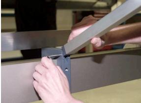
Step 5e - Align each Stand Bracket with a Rear Strut. Slip locking pin in place.
