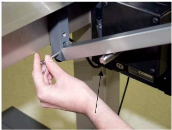
Step 8b - Align the Right Front Strut to the Right Stand Bracket. Secure with locking pin.
