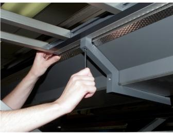
Step 9a - Align the Front Table Top to the Left Printer Bracket. Attach the Front Table Top to the bracket using a long screw. Repeat for remaining bracket.
