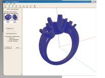
Optional ProtoWizard CAM software steps you through the model making process.
