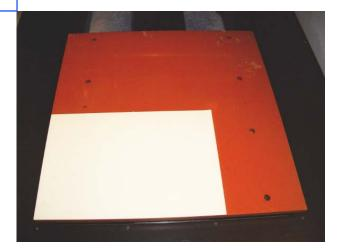
Please ensure the table is clean and free of debris. Remove protective AS-10 sheet coverings and place on table. Place the sheet on the lower left hand corner as we will be using that corner as our origin point.
