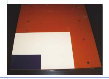
Place material on the lower corner and press onto sheet. The AS-10 sheet is a non adhesive reusable sheet and can be used several times before needing to be replaced.
