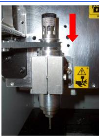
Gently install the tool and adaptor assembly from the top of the spindle assembly and turn counter clockwise to tighten. Only use finger pressure to tighten the assembly.
