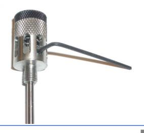
Install diamond scribe tool into spring loaded adaptor using included wrench.
