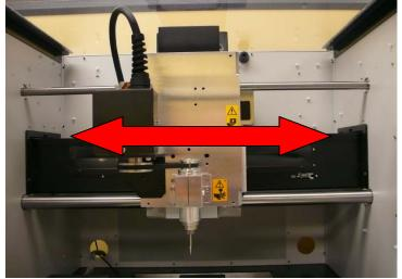
6. Clean guide rails and remove excess grease using lint free rag.
