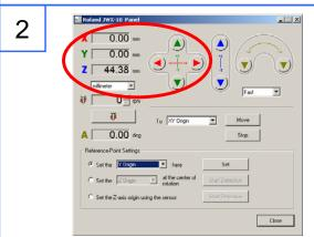
Move the tool to the X & Y Origin Position.
