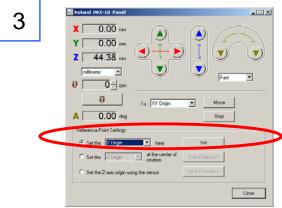
Set the Y-Origin at this location using the setting shown. After pressing the "Set" button, the Y-Origin will now read 0.00 mm.
