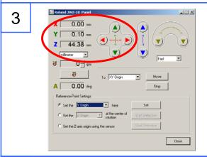
Move the tool half of the measured offset in the Y-direction only.
