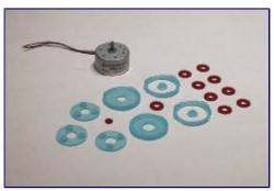
Zalewski decided to use a more revealing color scheme for the final assembly: a translucent turquoise body (solvent blue 70) with opaque, cerise gears (quinacridone pink). This photo shows all the parts with the post-casting film removed.
