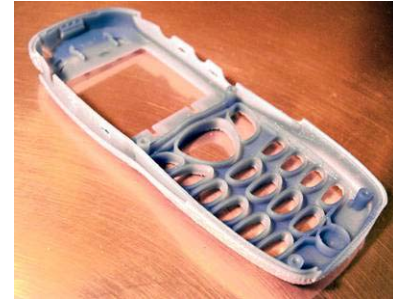
Figure 55 – The upfacing surface of the cell phone is smooth and highly detailed.
