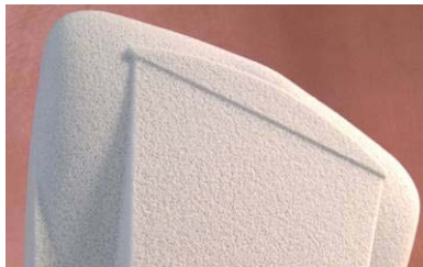
Figure 49 – Although there is no stair stepping, the light-density modeling board has a slight texture.
