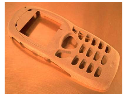
Figure 47 – Smooth surfaces and sharp detail from the MDX-650.
