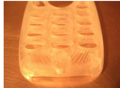
Figure 51 – Stair stepping is apparent on the shallow curve of the key pad area.
