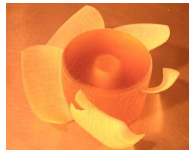
Figure 42 – Curled and damaged blades.
