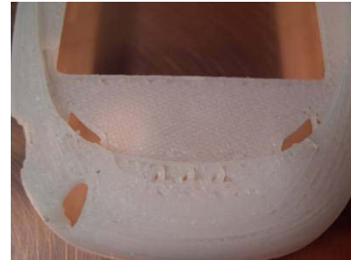
Figure 44 – Stair stepping and voids around small details.
