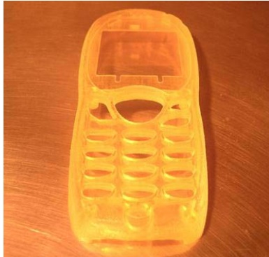
Figure 40 – The thin layers of the process offer smooth surfaces, even on the shallow arc of the key pad area.
