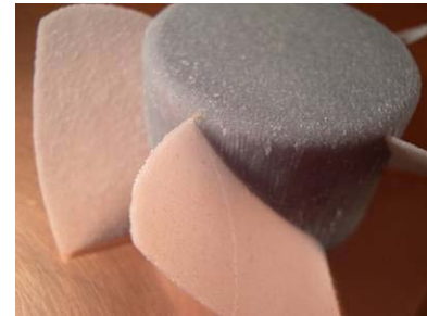
Figure 57 – In contrast to the smooth upfacing surfaces, the downfacing surfaces are rough.
