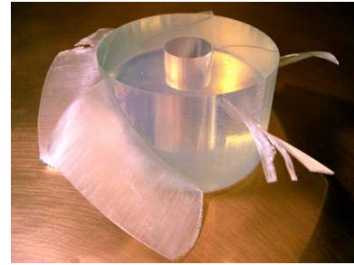
Figure 52 – Due to a support structure problem, the top edge of the fan blades curled and separated.
