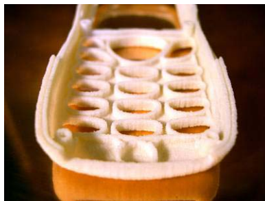
Figure 37 – The slots on the left and right sides are partially filled with excess powder.
