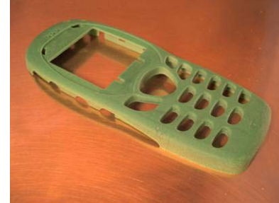
Figure 54 – Smooth surfaces and crisp details from the PatternMaster.
