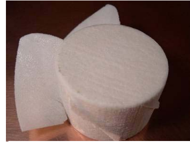
Figure 39 – Three of the fan blades detached during removal from the system.
