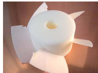
Figure 45 – With the exception of chipping during support removal, this fan was one of only two that would be suitable for prototyping applications.
