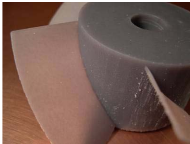
Figure 56 – Although the fan built successfully, the wax-like material was too fragile for routine handling.
