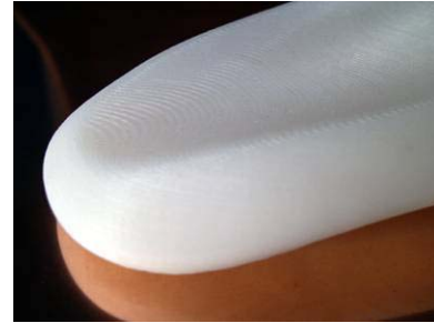
Figure 46 – While stair stepping is evident, it is less noticeable than expected.
