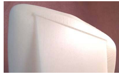
Figure 50 – The surface of the Delrin part is smooth and free of texture.
