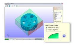
3. SRP Player automatically orients the part, generates toolpaths and provides you a finished preview. Just click Send to Machine to mill your finished part with smooth surfaces, tight tolerances
