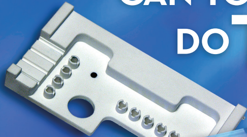
GLASS-TEFLON GUIDE PLATE Milled from glass-filled Teflon, providing mechanical strength and heat resistance up to 300° C.
