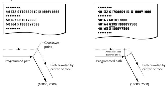
G39 is a word that is effective only within the block where it is specified. G39 functions only once, and circular interpolation is canceled in the next and subsequent blocks. G39 does not affect G00, G01, G02, or G03.
