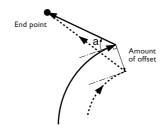
From an arc to a line (Type B)
