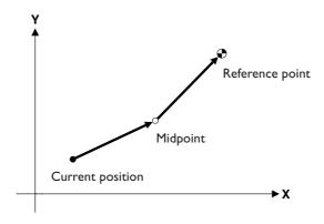
The midpoint is determined as follows. When X x, Y y, Z z is omitted, the coordinate of a G28 code executed in a previous block is used. Also, when no coordinate at all has been specified for a particular axis, no movement along that axis is performed. An example is shown below.
