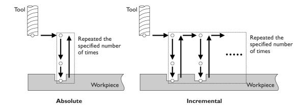
Fixed cycles can be used only with X-, Y-, and Z-axis coordinates. An A-axis coordinate cannot be included. Also, drilling can be performed only along the Z axis. Selecting the Y-Z plane or Z-X plane with G18 or G19 is not possible. None of the fixed cycles includes a function for starting the spindle motor. If the spindle motor is not already turning, an M03 word should be given beforehand to start rotation. Executing a fixed cycle while the motor is not rotating results in an error.
