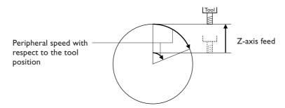
When the Z axis is at its highest position, the rotary axis unit rotates at maximum speed irrespective of any specified F code.
