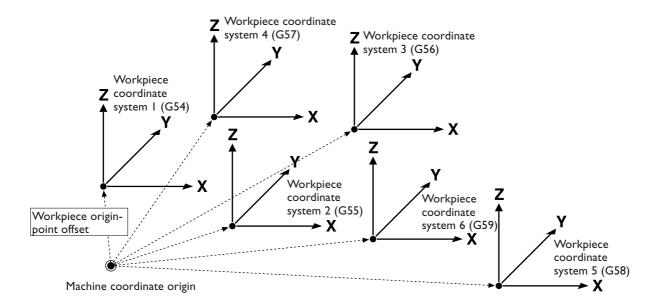
Note, however, that the state shown in the figure above is obtained when EXOFS is zero. EXOFS (the external workpiece origin-point offset) shifts the six workpiece coordinate systems as a group. The setting for EXOFS is made on the modeling machine. (It can also be specified using G10.)
