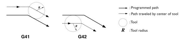
G41 or G42 is specified immediately after positioning (G00) or linear interpolation (G01). Tool-diameter offset cannot be started with circular interpolation (G02 or G03). Also, compensation on this machine is performed only for the X-Y plane, and so G17 (setting of the X-Y plane) is specified before G00 or G01.
