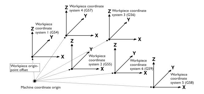
The locations of the six workpiece coordinate systems (that is, the six workpiece origin-point offsets) are set on the modeling machine.
