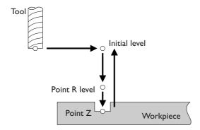
Cutting is performed at the spindle speed and feed rate that have been specified.
