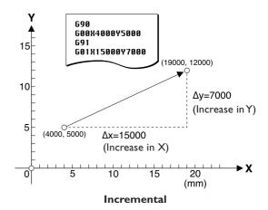
No special rules exist for deciding when to use an absolute or an incremental program. Examine the drawing and choose the one that makes for the simplest program.
