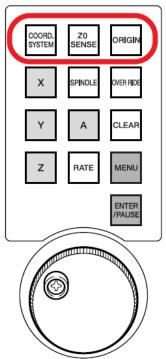
2. Select Z-Brake Check and press Enter. Once the Z-Brake is released, the Z-Axis will be free to be moved by hand as the X&Y axis are normally when the power is turned off.
