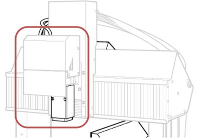
4. Press the Enter button on the Handy Panel. The Z-Axis can now freely move up or down.
