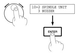
Turn the dial to move the arrow to [HIGH TORQUE] or [HIGH SPEED], then press the [ENTER] key.
