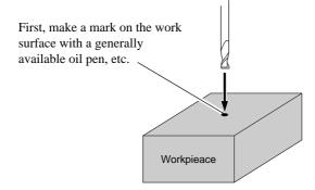
Press the [SPINDLE] key to make the spindle rotate. Place the tool in the marked position, then lower the tool until the ink is cut off. The ink mark on the work surface has a certain thickness, so only the ink is removed.
