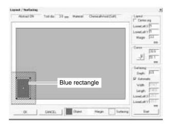
Double-clicking on one of the black circles displayed at the four corners of the object lowers the tool at that location. This lets you visually confirm the cutting location.
