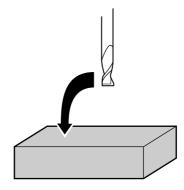
Turn the dial to align the tip of the cutting tool with surface of the workpiece.
