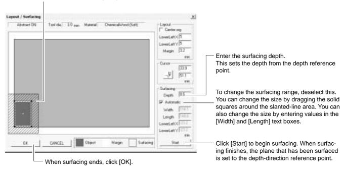
When surfacing finishes, MODELA Player and the coordinate view on the MDX-650/500 automatically sets Z0 on the surface of the workpiece after surfacing.
