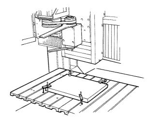
After cutting has finished, remove the cut material and load a new piece. Set the origin point if necessary.
