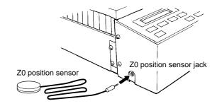
**9** Place the Z0 position sensor on top of the workpiece.
