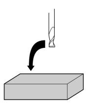
Turn the dial to gradually move the cutting tool to the height where the Z1 point is to be set.
