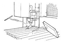
Align the pin on the back of the spindle unit with the pinhole on the slider, and support it with your hand.
