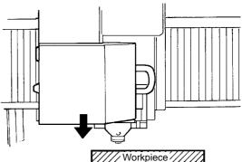
Insert the cutter into the hole in the cutter holder and position the tip so that it gently touches the surface of the workpiece. Use the hexagonal screw driver included with the ZC-500TE to tighten the screw.
