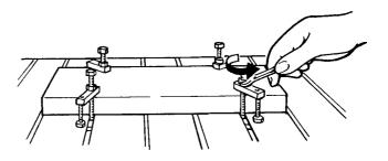
Turn the large bolts as shown in the figure to align the workpiece-side end of the clamp with the height of the secured portion.
