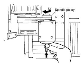
Use the included wrenches to tighten the spindle pulley and collet (150 to 200 kgf·cm).
