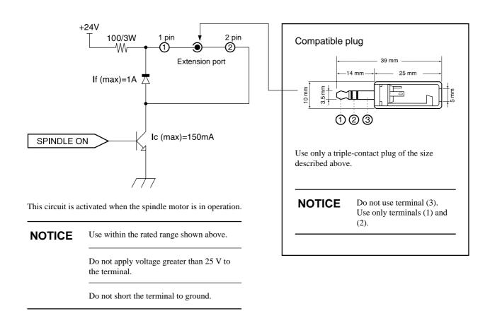
No responsible is assumed for effects to which any equipment connected to this external output connector is subjected.
