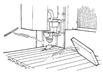
Align the pin on the back of the spindle unit with the pinhole on the slider, and support it with your hand.
