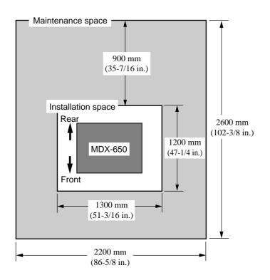
When you are installing the MDX-650 on a stand, use a stand with specifications equivalent to those shown below.
