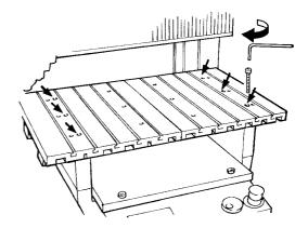
Align the T-slot table removed in step 3 with the pinholes on the spacers and set into place.
