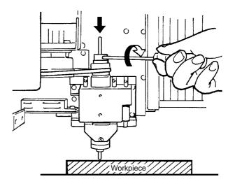
Use the operation panel to set the Z-axis origin point. The Z-axis origin is the reference point for raising and lowering the spindle. For information on how to make the setting, refer to User's Manual 2 or User's Manual 3, depending on the command set you're using.
