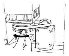
Pass the belt through under the motor pulley and engage on the spindle pulley.
