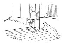
**NOTICE** When mounting a vise or loading a workpiece while a tool is installed, take care to avoid being injured by the tool.
