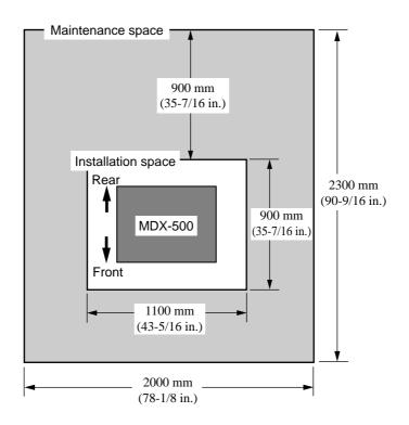
When you are installing the MDX-500 on a stand, use a stand with specifications equivalent to those shown below.
