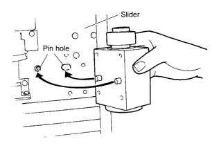
**2** Insert the screw at the location shown in the figure, then tighten using the included hexagonal screwdriver.
