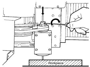
Use the operation panel to set the Z-axis origin point. The Z-axis origin is the reference point for raising and lowering the spindle. For information on how to make the setting, refer to User's Manual 2 or User's Manual 3, depending on the command set you're using.
