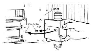
**2** Insert the screw at the location shown in the figure, then tighten using the included hexagonal screwdriver.
