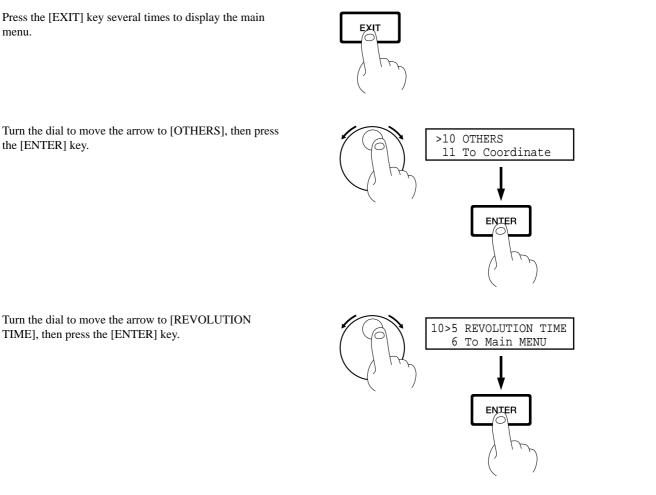
Turn the dial to move the arrow to [REVOLUTION TIME], then press the [ENTER] key.
