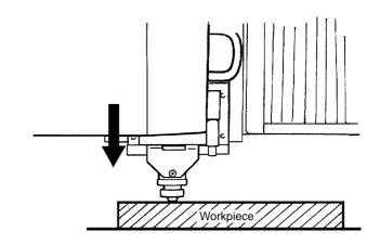
If the depth regulator nose does not reach the surface of the workpiece even when the tool down (-Z) key is held down, rotate the micrometer dial in the direction shown by the arrow in the figure to extent the tip of the depth regulator nose to the workpiece surface.
