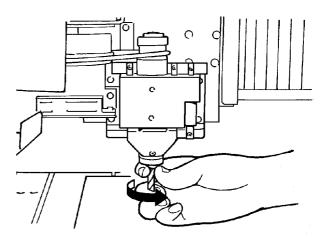
Spindle pulley Wrench (10 mm(3/8 in.))
