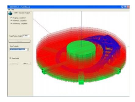
Finish Toolpath is radial for shorter machine time and better detail finish...
