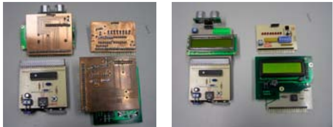
Students at Victoria University's Electrotechnology and Computer Systems Department design and produce their own custom PCBs using Roland MDX-20 scanning and milling machines.
