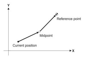
The midpoint is determined as follows. When  $\mathbf{X} x$ ,  $\mathbf{Y} y$ ,  $\mathbf{Z} z$  is omitted, the coordinate of a G28 code executed in a previous block is used. Also, when no coordinate at all has been specified for a particular axis, no movement along that axis is performed. An example is shown below.
