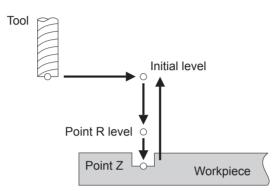
Cutting is performed at the spindle speed and feed rate that have been specified.
