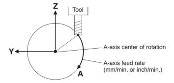
The speed of rotation of the A-axis varies according to the position in the Y- and Z-axis directions. Note, however, that the situation just described occurs when the Y- and Z-axis origins are at the A-axis center of rotation and the Y- and Z-axes are both at rest. It is important to note that performing simultaneous feed of the Y and A, Z and A, or Y, Z, and A axes does not result in the intended speed.
