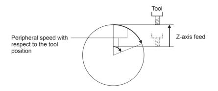
When the Z-axis is at its highest position, the rotary axis unit rotates at maximum speed irrespective of any specified F code.
