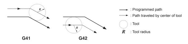
G41 or G42 is specified immediately after positioning (G00) or linear interpolation (G01). Tool-diameter offset cannot be started with circular interpolation (G02 or G03). Also, compensation is performed only for the X-Y plane, and so G17 (setting of the X-Y plane) is specified before G00 or G01.
