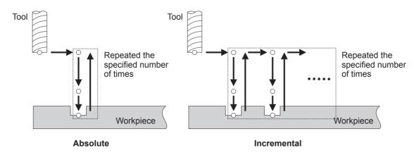
Fixed cycles can be used only with X-, Y-, and Z-axis coordinates. An A-axis coordinate cannot be included. Also, drilling can be performed only along the Z axis. Selecting the Y-Z plane or Z-X plane with G18 or G19 is not possible.
