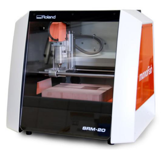
Accessories included in the box: ZC-20-32 (Bottom Load 1/8" Collet) ZC-20-60 (Bottom Load 6mm Collet) ZHS-3015 (Endmill 3mm straight end mill with a 6mm shank) EMF-125-2F-125 (1/8" Shank, 2 Flute, 1/8" Mill, 0.375" Flute Length, 1.5" OAL) \*\*\*
