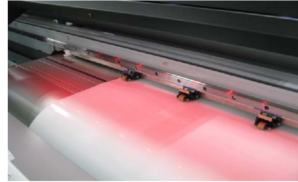
LED on top turns on RED If a service call or motor error occurs
