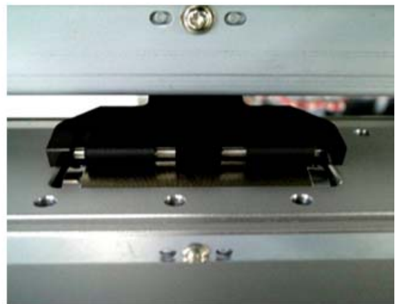
New Pinch Roller Assembly (22 rollers - XJ-540, 26 rollers - XJ-640, 30 rollers - XJ-740).
