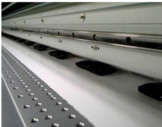
New Pinch Roller Assembly (22 rollers - XJ-540, 26 rollers - XJ-640, 30 rollers - XJ-740).
