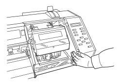
Pull out the carriage in the direction shown in the figure.
