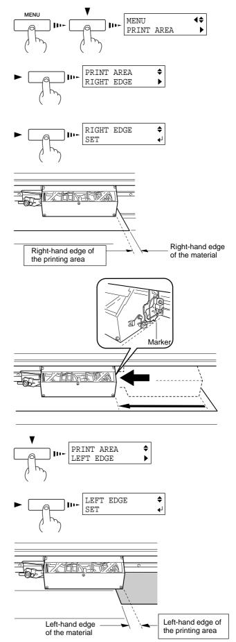
Use the [ ◀] and [ ▶] keys to move the marker at the right edge of the carriage to the location you want to make the left edge of the printing area. Press the [ENTER] key to lock in the setting the left-hand edge with an audible beep.
