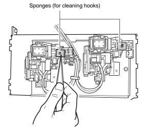
Orient a new sponge (included with the cleaning kit) as shown in the figure (lengthwise) and insert it.
