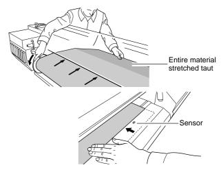
With the material pulled out from the roll stretched taut with no slack, move the sheet loading lever toward LOAD.
