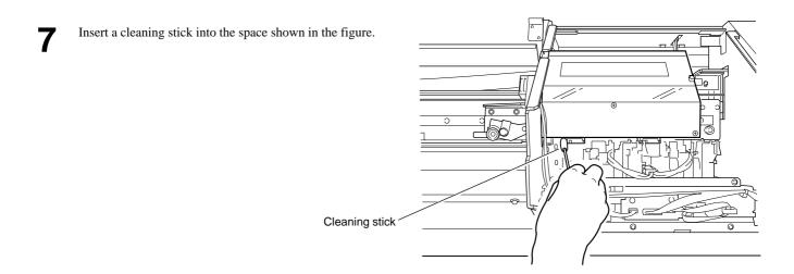
Move the carriage to a location where the cleaning stick reaches the left-hand side surface of the left-hand head, and wipe away any grime on the left-hand side surface (the metal area) of the left-hand head.
