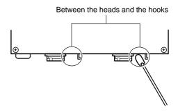
Pull the carriage by hand to move it to the left-hand side until the black rubber caps, sponges, and tubes can be seen.
