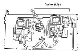
20 Clean the wiper areas (two places on the left and right). When viewed from the front, the wiper has a rubber surface on its right-hand side and a felt surface on its left-hand side. Clean mainly the rubber surface and the top edge.
