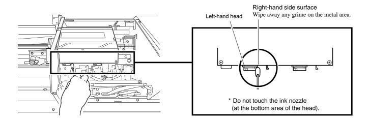
Move the carriage to a location where the cleaning stick reaches the front surface of the left-hand head.
