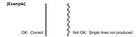
If misalignment like in the example occurs when the printing direction for [PRINT QUALITY] has been set to [BI-DIRECTION] (bidirectional), then carry out correction at the [BIDIRECTION] menu (see "2-5" Printing - Making Corrections for Printing - Bidirectional Correction").
