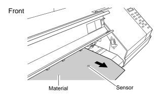
Grasp the front edge of the material at the front of the machine and turn the media flanges at the back of the unit to roll back the media.
