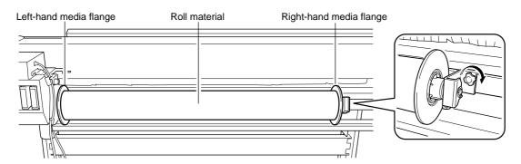
Pass the end of the material through the unit from back to front.
