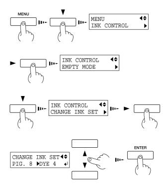
When the display shown in the figure appears, discard the discharged ink in the drain bottle.
