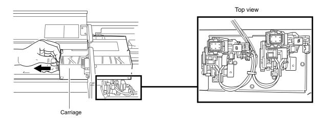
Wipe away any grime adhering to the edges of the left-hand and right-hand rubber caps. Use the tip of the cleaning stick to scrape off grime.
