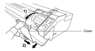
To discharge static electricity from your body, touch the location shown in the figure.
