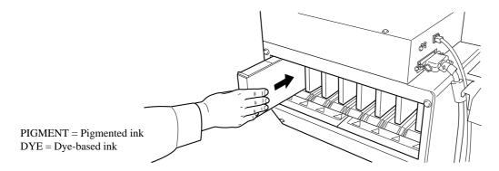
Before you insert a cartridge, make sure the ink color matches the slot where it is to be inserted.
