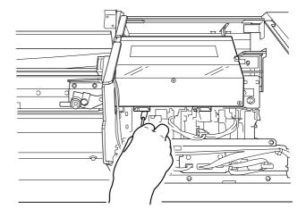
Move the carriage to a location where the cleaning stick reaches the back surface of the left-hand head.
