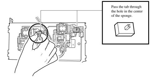
Orient as shown in the figure (lengthwise) and attach it, being careful to hold it straight as you do so. There is no distinction between left and right or between front and back.
