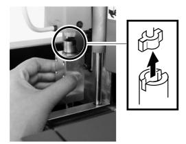
While supporting the spindle by hand, use the included hexagonal (large) wrench to loosely tighten the screws you removed in step 1.
