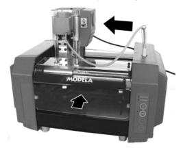
Hold down the TOOL-DOWN key to lower the blade to close to the surface of the workpiece.
