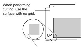
The center of the hole at the lower left of the work plate is the suggested X- and Y-direction machining reference point for Modela.
