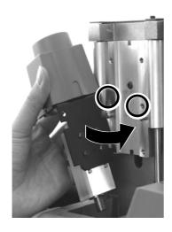
Insert the screws at the locations shown in the figure, and tighten them loosely using the included hexagonal wrench (large). After attaching all two screws in this way, tighten them securely.
