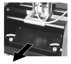
Install the work plate on MODELA and tighten the screws
