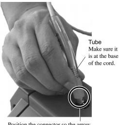
Position the connector so the arrow points to the back of the unit and insert.
