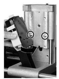
Insert the screws at the locations shown in the figure, and tighten them loosely using the included hexagonal wrench (large). After attaching all four screws in this way, tighten them securely.
