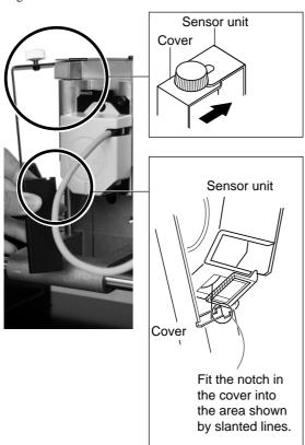
While gently pressing down on the cover with one hand, tighten the screws shown in the figure.
