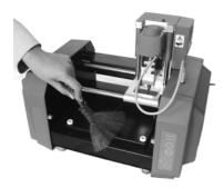
Lift up MODELA and also remove any cuttings that may have fallen underneath.
