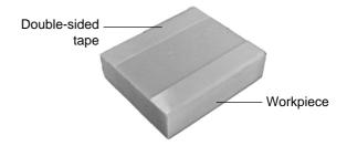
Mount the workpiece with its corner aligned with the position of the work plate in the figure.
