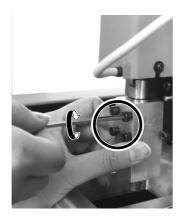
Pull out the spindle from below to remove it.
