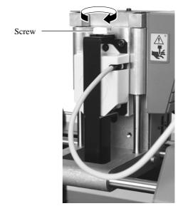
Remove the sensor unit by following steps 2, 3, and 4 of "Installing the Sensor Unit" in reverse order.
