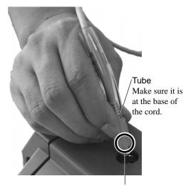
Position the connector so the arrow points to the back of the unit and insert.
