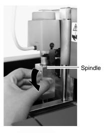
Insert the blade shank into the spindle.
