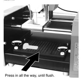
Orient so the surface with the grid faces up.
