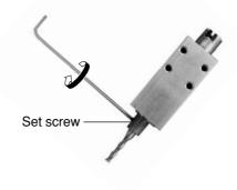
Fit the spindle into place as shown in the figure.
