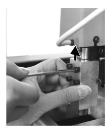
lift up the spindle until it touches, and while holding the spindle in that position, use the included hexagonal (size: 3 mm) wrench to loosely tighten the screws you removed in step 1.
