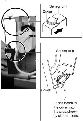
While gently pressing down on the cover with one hand, tighten the screw shown in the figure.
