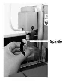
Insert the blade shank into the spindle.
