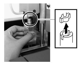
After all four screws are in place, While supporting the spindle by hand, tighten securely.
