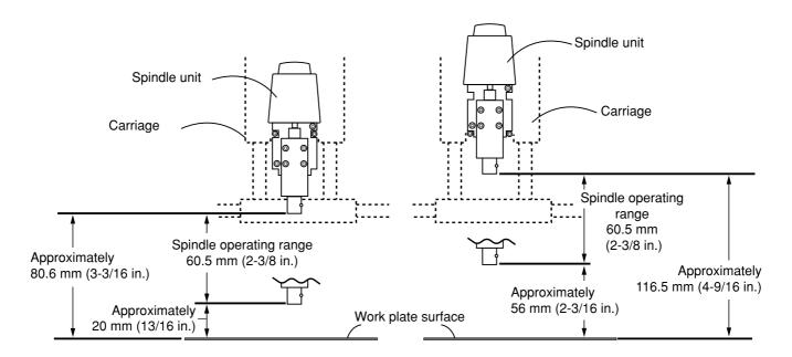
Load the material and install the tool. When using a base to load the material, mount the base as well. Make the layout the same as for actual cutting.
