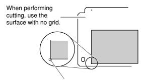
The center of the hole at the lower left of the work plate is the suggested X- and Y-direction machining reference point for Modela.
