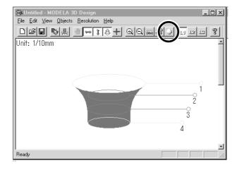
Drag the scroll box for the X, Y, or Z scroll bar. The object rotates, letting you view it from various perspectives. To color the object, click [Start].
