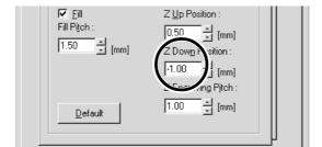
For [Fill Pitch], enter the diameter of the tool tip.
