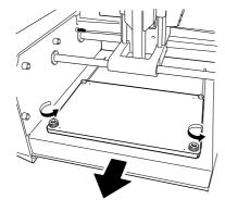
Install the work plate on MODELA and tighten the screws.
