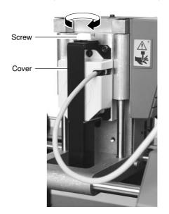
Remove the sensor unit by following steps 2, 3, and 6 of "Attach the Sensor Unit" in reverse order.
