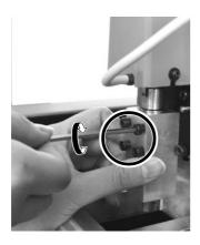
**9** Pull out the spindle from below to remove it.
