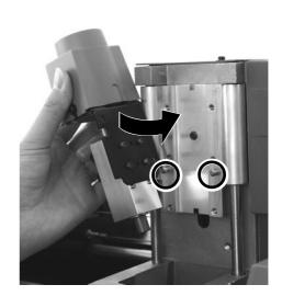
Insert the cap screws at the locations shown in the figure, and tighten them loosely using the included hexagonal wrench (size: 3 mm). After attaching all two screws in this way, tighten them securely.
