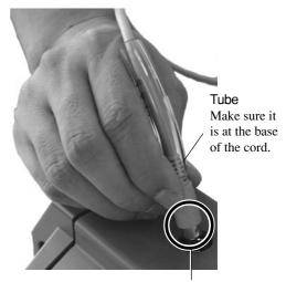
Position the connector so the arrow points to the back of the unit and insert.
