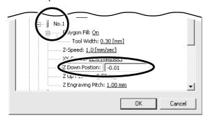
For [Fill], click [Tool Width], then enter the diameter of the tool tip.
