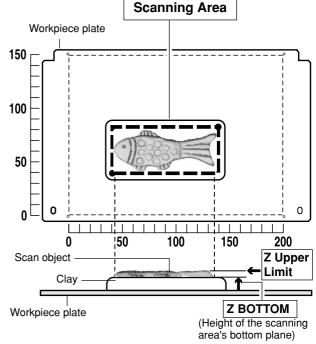
\* If you have made a clay base, the height of the clay is taken to be the Z-axis reference surface.
