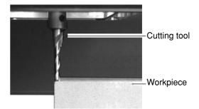
Lower the tool at the four remaining corners with the new reference point, and make sure that the material is not cut. (See "2. Verify the Cutting Position and Height When the Tool Is Lowered" in the previous section.) If the material is cut, then repeat steps 2 and 3 and set a new reference point.
