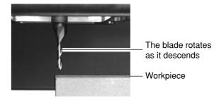
When the blade tip comes close to the material surface, carefully use the key to lower the blade a little at a time.
