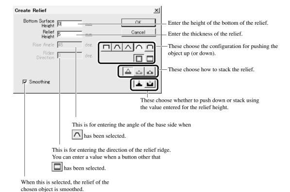
The display changes automatically to the screen at right, and a three-dimensional view of the shape of the relief appears.
