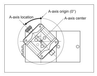
The location of the A-axis is indicated as an angle of rotation. In this way it differs from how the X-, Y-, and Z-axes are indicated. Despite this difference between angles and distances, in other respects it is treated the same as X-, Y-, and Z-axes coordinates. As with any of the other axes, you can freely set location of the origin (despite it being an "angle" and not strictly a "point") and select the coordinate system.
