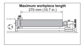
The length of a workpiece that can be loaded is as indicated left. If an item exceeds this, contact with the live center is impossible.
