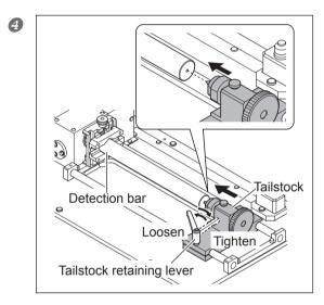
Loosen the tailstock retaining lever, move the tailstock, and make the end of the live center hit against the hole on the center of the detection bar.
