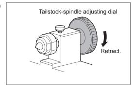
Turn the tailstock-spindle adjusting dial and retract the tailstock spindle.
