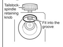
The tailstock-spindle adjusting dial may run idle and it may not be possible to remove the live center. In this case, the end of the tailstock-spindle retaining knob is dislocated from the groove of the tailstock spindle. Adjust the position so that the end of the tailstock-spindle retaining knob fits into the groove of the tailstock spindle, and then turn the tailstock-spindle adjusting dial.
