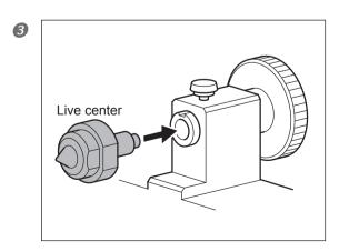
Insert the live center (or the center drill) into the hole of the tailstock spindle.
