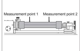
As the diagram on the left shows, determine two arbitrary measurement points on the same surface of the workpiece and make a mark.
