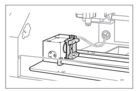
Rotate the A-axis by manual feed so that the vise tightening knob is above the A origin.
