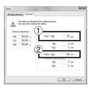
Enter the X-axis coordinate at Measurement 1 and 2, which were recorded at step 4.
