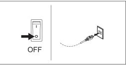
Turn off the modeling machine and unplug the power cable.
