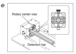
Install the detection bar to the rotary center vise.
