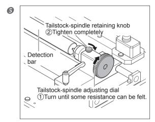
①Turn the tailstock-spindle adjusting dial towards the arrow direction until some resistance can be felt.
