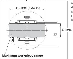
Make sure that the corner of the workpiece does not exceed the maximum workpiece range. For example, when you're using square material whose height is 40 millimeters (1.57 in.), the maximum depth is 110 millimeters (4.33 in.).
