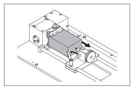
Detach the center drill from the workpiece.
