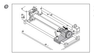
Open the front cover. Turn the tailstock retaining lever to move the tailstock.
