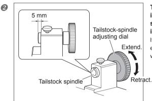
Turn the tailstock-spindle adjusting dial and protrude the tailstock spindle about 5 millimeters (0.197 in.).
