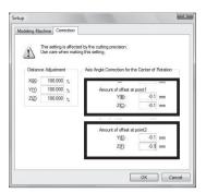
Enter the displacement amount of Y- and Z-axis coordinates at Measurement Point 1 and 2.
