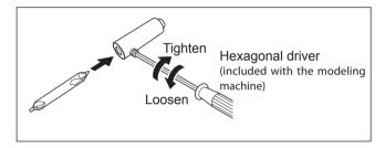
The center drill is fitted with a bit at each end. When the one in use becomes worn, reverse the orientation and reinstall. When both ends become worn, then replace.
