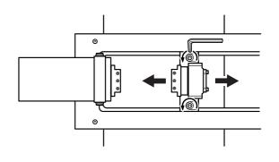
Use the included hexagonal wrench (3 mm) to loosen the set screws for the workpiece retainer attachment on the drive and support sides, then insert the workpiece.If the workpiece is flat, press the flat surface of the workpiece against the workpiece brace surface of the workpiece retainer attachment.
