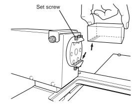
Tighten the set screws securely, using even force. If the workpiece is thin and the set screws do not reach, insert the included spacer or the like and secure in place.
