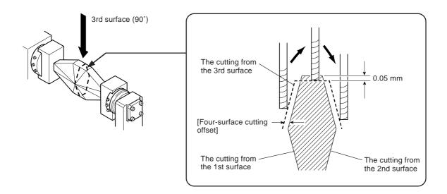
This actively uses the bottom surface of the tool (the bottom tool) by cutting deeply. It also uses [Four-surface cutting offset] to make the tool move away toward the outer side to keep the side of the tool (the outer peripheral tool) from touching surfaces that have already been finished. You can adjust [Four-surface cutting offset] to match the size of the error in accuracy.
