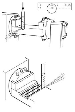
Use the  $[\blacktriangle], [\blacktriangledown], [\blacktriangleleft]$ , and  $[\blacktriangleright]$  keys to move the tool, then cut the workpiece. Cut a sufficient range to allow use of Vernier calipers or the like.
