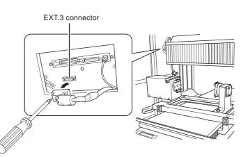
Firmly insert the ZCL-650 cable into the "EXT.3" connector on the MDX-650. Use a screwdriver to tighten the connector screws. The ZCL-650 will not operate if this cable becomes disconnected or loose. Tighten securely.
