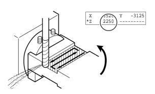
Use the coordinates a and b that you noted in steps 4 and 7 to calculate the theoretical value for the finished thickness. Also, use Vernier calipers or the like to measure the actual thickness of the cut workpiece. The difference between the theoretical value and the actual measured value is the amount of error. As a general guide, the offset value should be one-half of this.
