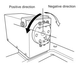
Holding down the [JOG] key again for 0.5 seconds or longer changes from the A axis to the Y axis.
