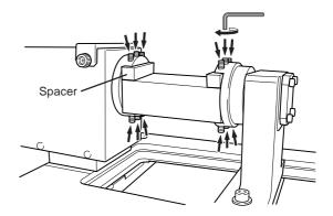
Take care not to apply excessive force when securing the workpiece in place. Doing so may cause the workpiece to warp or deform during cutting. When you are using a soft workpiece made of foamed material or the like, precision may be affected by slipping of the workpiece during cutting or twisting during rotation.
