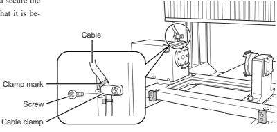
If you're using the optional safety cover (ZBX-650), remove the plate on the left side of the ZBX-650.
