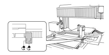
Use two screws to attach the cable clamp and secure the cable in place. Position the cable clamp so that it is between the white clamp marks.
