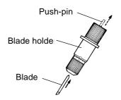
Adjust the amount of blade extension as shown in figure to find the optimal amount of blade for the target material.
