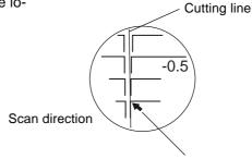
Read the scale on which the cutting line goes over as the correction-value .
