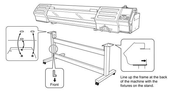
**Q** Use the included large bolts to secure the machine to the stand.
