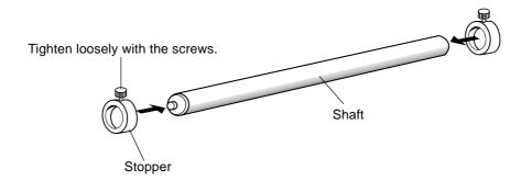
Attach the two shafts and engage the brake. Install the shafts so that the one with the stopper is in front of the back of the machine.
