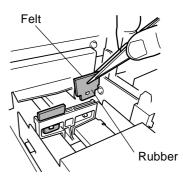
Install the new wiper.Use the tweezers to press the
