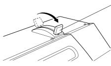
To secure the media in place, move all the way to "LOAD".
