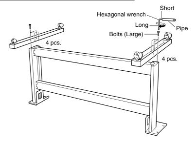
2 Set the stand upright so that the casters are at the bottom, and place the machine on the stand. The front and rear of the stand are as shown in the figure.
