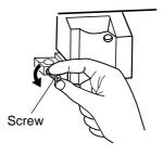
6 Support the tool-securing screw from below and install the blade holder.
