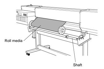
When viewed from the front, align so that the left-hand edge of the media is above any of the grit rollers and the right-hand edge is above any of the three grit rollers of the right side of the main unit.
