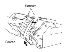
6 To discharge static electricity from your body, touch the location shown in the figure.
