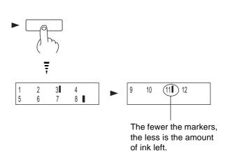
3 Continuing by pressing the [ ▼ ] key lets you check the amount of remaining ink for ink cartridges 9 through 12.
