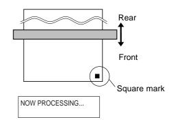
While automatic adjustment is in progress, the following message appears on the display.
