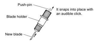
6 Support the tool-securing screw from below and install the blade holder.
