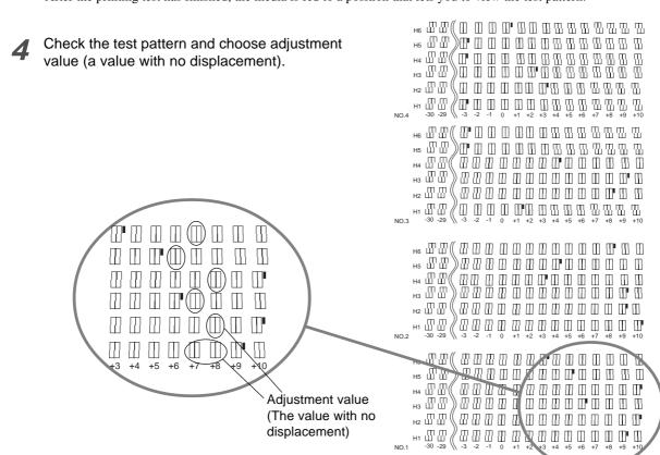
**5** Check the adjustment value, then press the [ENTER] key. The media returns to its position when the printing test ended.
