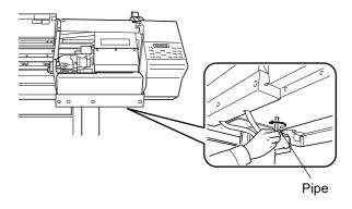
Align the guides at the two ends of the cap unit with the guides at the two ends of the printing carriage.
