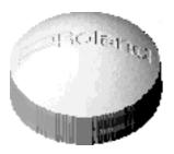
Make sure the item to be engraved is made of a material that your modeling machine can cut. This example uses chemical wood.
