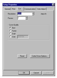
Resolution- Determines how closely the knife follows the lines. Higher settings increase accuracy.
