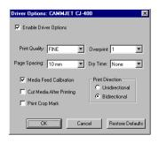
When this option is checked, the settings made in this dialog are sent to the printer, overriding temporarily the settings made through the printer panel. When it is unchecked, the settings in the printer panel are used.
