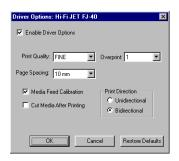
By checking Enable Driver Options, printer-specific options defined here are sent to your printer to override option settings currently made through your printer menu. When it's unchecked, the printer settings are used.
