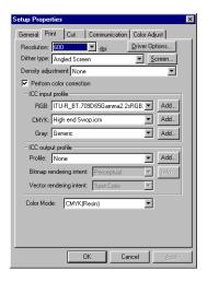
**Resolution-** You may set the output resolution here. A higher resolution will generally result in better results but slower output. The resolution set here is separate from the resolution used by your application.
