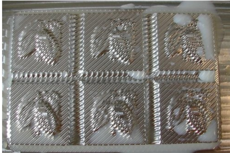
Mold plate assembly machining
