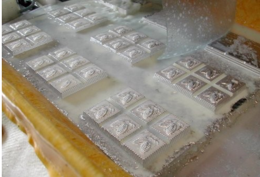
Mold plate assembly machining
