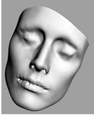
Fast Skin Method: The boundary curves of 4 surfaces (left) were sketched easily to calculate NURBS surfaces (right). The result of such fast and simple method may create ripples (see the mouth).
