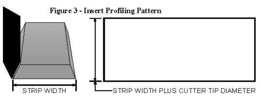
pattern must be created that will yield a plate the proper length and width. A simple rectangle is all that is needed (Figure 3).
