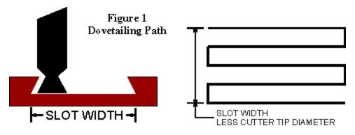
are using a .250" dovetail cutter. Since the lines of our logo pattern define the center of the cut - not the edge - we must subtract the cutter tip diameter from the finished slot width. In this case, 1.0" (slot width) minus .250" (cutter width) give us a pattern width of .75".
