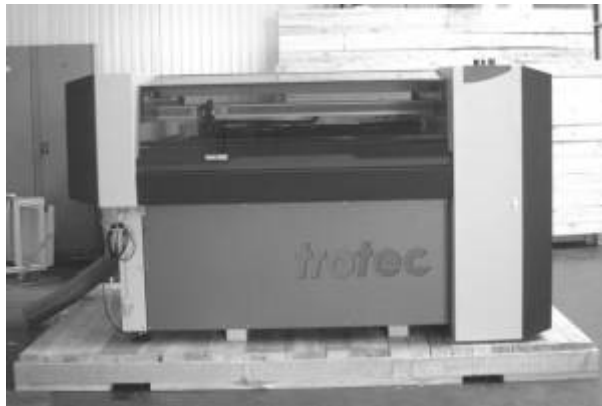
Photo 1: the Professional kept in position by wooden spacers
