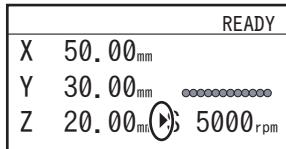
If no operations are performed for a certain amount of time and the cursor disappears, press [SPINDLE] several times to move the cursor to [S], and then operate the [Dial].
