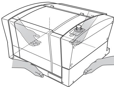
The weight of the machine alone is 35 kg (77.2 lb.). Unload and place the machine with care.
