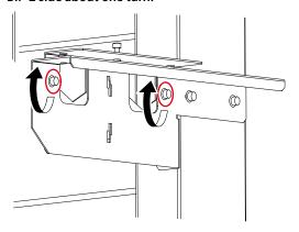
13. Perform adjustment by turning the adjustment screw
