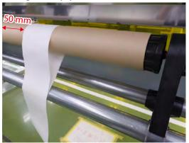
5. Insert the end of the paper ring between the grit roller and the pinch roller.
