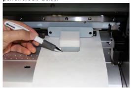
11. Measure the gap between the two lines with a ruler (the line you drew on the panel side and the line you drew on the BIF-2 side). If the gap is less than 1 mm, the adjustment of the feed adjuster is not necessary.
