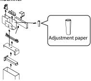
2. Roll the adjustment paper and make a ring. Then, put masking tape on both the inside and outside of the ring to secure it.
