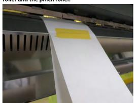
**6.** Pull the end of the paper ring for adjustment straight to the direction indicated by the red arrow.
