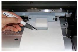
**9.** Move the paper ring for adjustment toward the BIF-2 side (Place it approx. 50 mm from the right edge of the paper tube).
