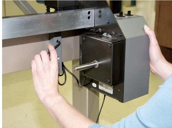
Step 6a – From the front of the printer, lock down the Stand Brackets. Apply only enough turns to keep the Stand Bracket from moving.
