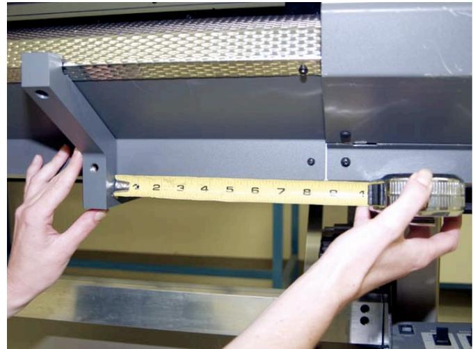
Step 7c - Measure or estimate 8.5 from right edge of the Printer Apron. Lock down the remaining Printer Bracket just enough to hold the bracket in place.
