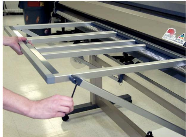
**Step 8f - Place Front Table Top onto Printer Brackets or Printer Apron. Attach each strut to the Front Table Top with long screws.**
