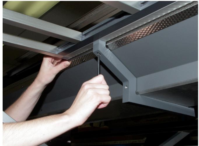
**Step 9a - Align the Front Table Top to the Left Printer Bracket. Attach the Front Table Top to the bracket using a long screw. Repeat for remaining bracket.**
