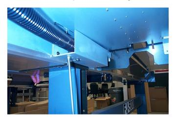
10. Unlatch and slide the main harness inside the second large clamp and latch in place.
