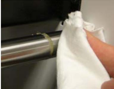
7. Reapply a small amount of grease on finger and spread a **light** coating on the guide rails.
