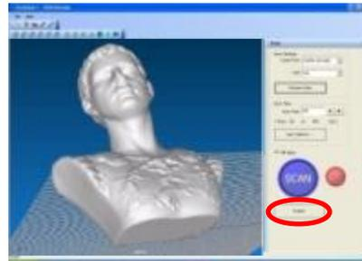
Point cloud data is automatically cleaned and converted to polygon data
