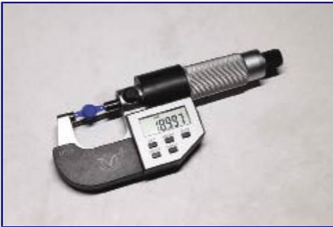
Measurement taken after post-cure. Original CAD dimensions of this part: 19.000 mm. In general, accuracy better than 0.005 mm (0.0002 in.) can be expected if the process is carried out right.
