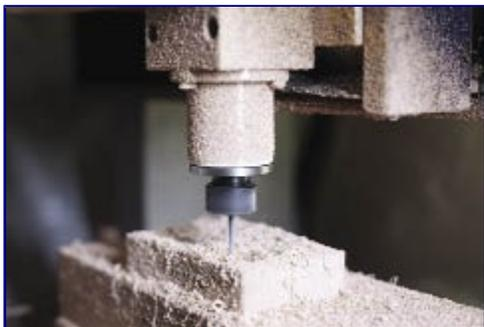
Rough machining of the mold for gearbox components on Roland Modela MDX-540 in Huntsman RenShape 460 prototyping board, with a 3 mm diameter square end mill at 12,000 RPM. This step took about 30 minutes to complete.
