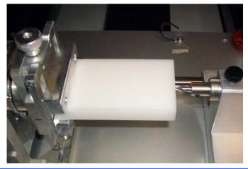
Place material into the self centering clamp. Install center drill and place next to end of material. The center drill will be used to place a small hole for the live center to placed into.
