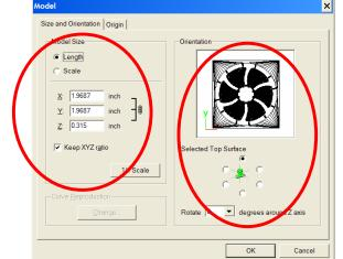
Check the size of the part as well as the orientation of the part. The view in the orientation window is from the top. If you need to change the orientation of the part, you would select the different surface view below the orientation view
