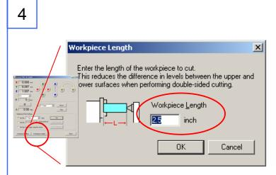
Click on the Workpiece length and enter the length of your material stock. Click **OK** when finished
