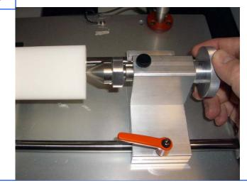
Move the live center support until the live center is touching the material stock. Turn the core support adjuster to ensure that the material is firmly supported. Turn the black adjuster lock to lock the core support adjuster.
