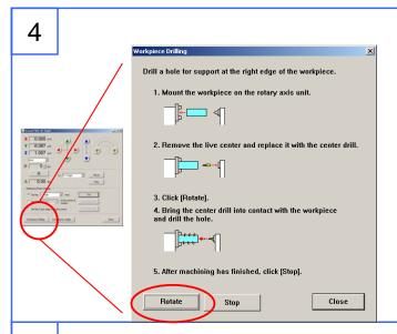
From the Virtual Control Panel, Click on the "Workpiece Drilling" Function. Click on the Rotate button to start the A-Axis spinning. Please make sure the machine is not in "view" mode.
