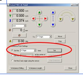
Set the X Origin by selecting the **Reference Point Settings** and selecting **X Origin**, and clicking on Set to set the X Origin. You will notice that the Virtual Control Panel will now display X 0.00.
