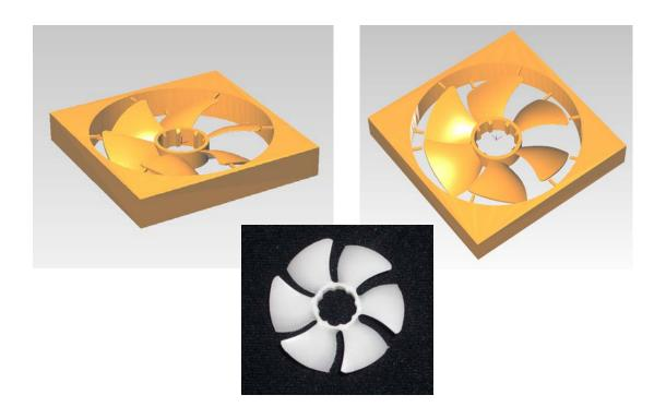
This tutorial will guide you through the various steps required of producing a double sided part using the MDX-40, ZCL-40, and Modela Player 4. The resulting functional part is a fan that can be used to blow chips away from the cutting surface.
