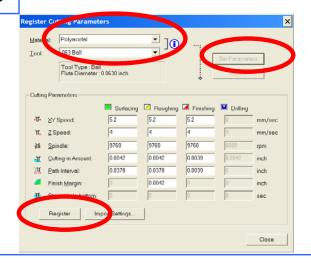
Select **Polyacetal** under Material (same as Delrin, acetal), click on **Set Parameters**, and **Register** to accept the cutting parameters.
