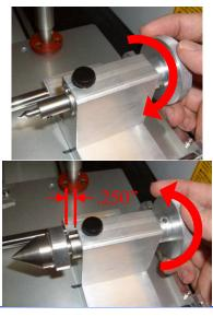
Remove the center drill by turning the core support adjuster until the center drill is free.
