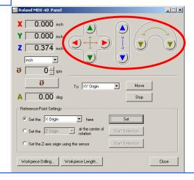
You will use the Virtual Control Panel to move the machine in the X,Y, Z, and A direction. You will also use this to set the various origins.
