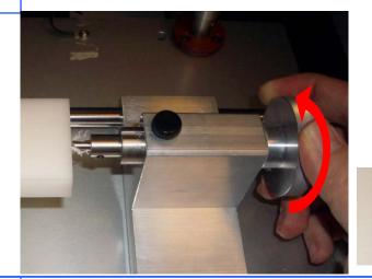
As the A-Axis rotates, **slowly** feed the center drill deeper into the part by turning the core support adjuster on the 4<sup>th</sup> axis support. Press the stop button when the drill cone is about half ways in the material.
