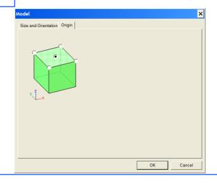
Click on the **Origin** tab and select the center of the part as the new origin. Click **OK** when finished.
