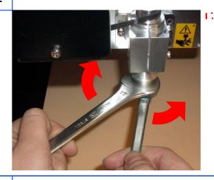
Install the collet and tool in the spindle. Place the 17mm tool in your left hand 1<sup>st</sup> and over the spindle nut as shown. Place the 10mm tool in your right hand and over the collet. To tighten, pull the wrenches away from each
