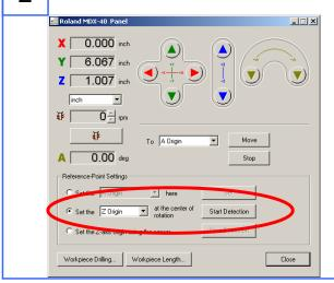
Select the **Z-Origin** for the "Set the Z-Origin at the center of rotation" reference point settings. Click on the **Start Detection** button. The Tool will move down, touch the Tool Sensor several times, and the Z-Origin will be set after this.
