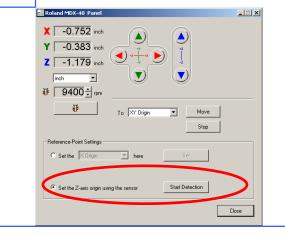
Select the **Z-Axis Reference Point Settings** and Click on the **Start Detection** button. The Tool will move down, touch the Tool Sensor 3 times, and the Z-Origin will be set after this. **Remove Tool Sensor.**
