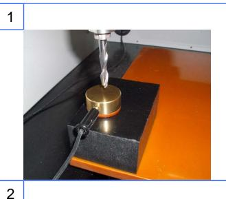
To set the tool Z-Origin on the top surface of the material, use the Tool Sensor and the place it over the material. Use the Virtual Control Panel to move the tool over the tool sensor.
