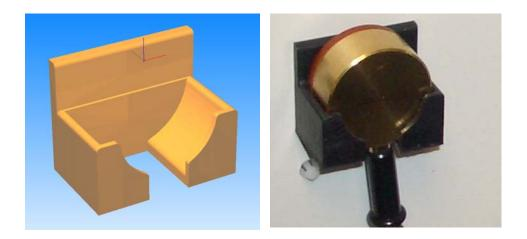
This tutorial will guide you through the various steps required of producing a single sided part using the MDX-40 and Modela Player 4. The resulting part is a tool sensor holder that can be used to hold the sensor in a safe, accessible location.
