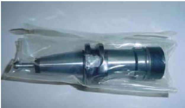
2. Apply silicone spray on the Tool Holder and wipe it clean.
