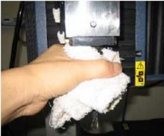
3. Press the [CLEAR] button to do a force release and hit the root of the tool holder from its front with a plastic hammer lightly.
