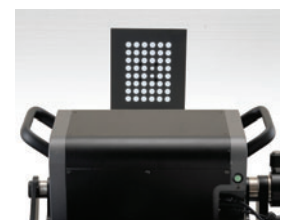
Compact calibration chart (standard accessory)
