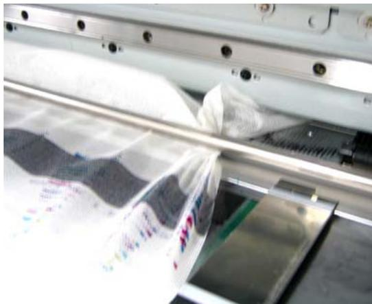
**Media feeding stops on the dryer due to clinging onto it. It causes wrinkling between Grit Roller and Tension Roller, while Grit Roller keeps feeding the Media.**
