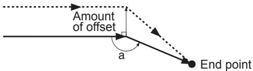
From an arc to a line (Type A)
