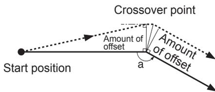
From a line to an arc (Type B)
