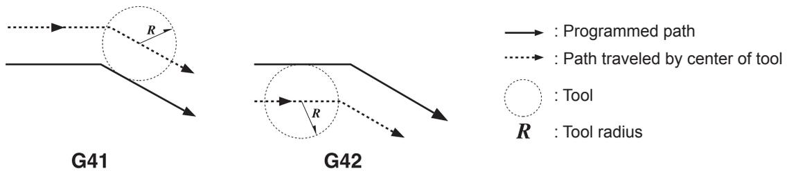
G41 or G42 is specified immediately after positioning (G00) or linear interpolation (G01). Tool-diameter offset cannot be started with circular interpolation (G02 or G03). Also, compensation is performed only for the X-Y plane, and so G17 (setting of the X-Y plane) is specified before G00 or G01.
