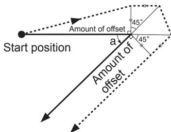
From a line to an arc (Type B)
