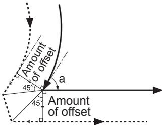
From an arc to an arc
