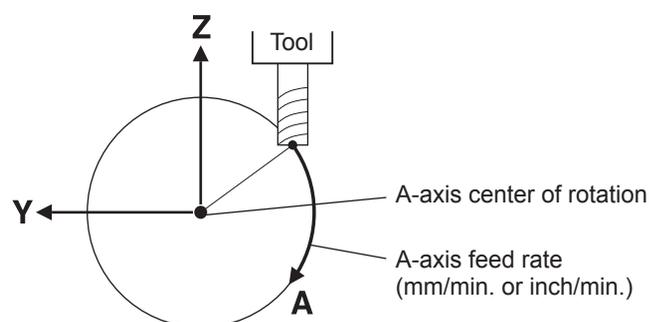
The speed of rotation of the A-axis varies according to the position in the Y- and Z-axis directions. Note, however, that the situation just described occurs when the Y- and Z-axis origins are at the A-axis center of rotation and the Y- and Z-axes are both at rest. It is important to note that performing simultaneous feed of the Y and A, Z and A, or Y, Z, and A axes does not result in the intended speed.
