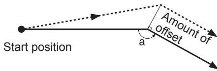
From a line to an arc (Type A)
