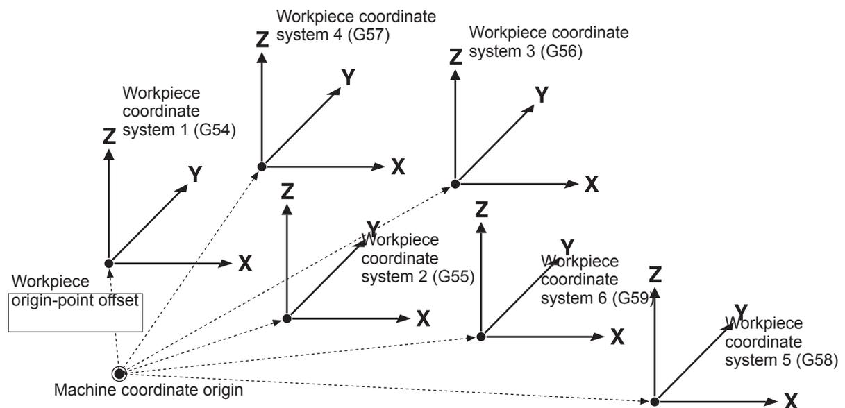
On a modeling machine equipped with a rotary axis unit, the A axis is added to this. The workpiece origin-point offset for the A-axis coordinate is expressed as an angle.
