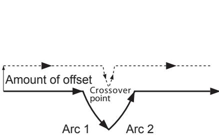
In this case, a crossover point exists on the tool path for arcs 1 and 2.
