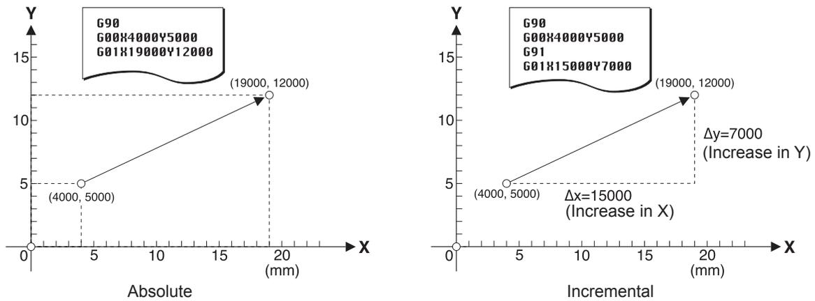
No special rules exist for deciding when to use an absolute or an incremental program. Examine the drawing and choose the one that makes for the simplest program.
