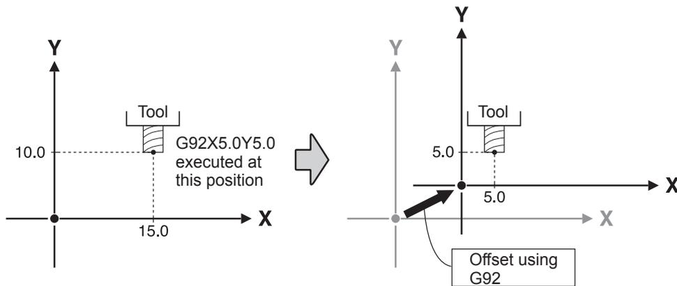
G92 calculates the offset value from the currently selected workpiece coordinate system (one of G54 through G59) and the current tool position. This offset value is then added to the respective workpiece origin-point offsets. That is, workpiece coordinate systems 1 through 6 are all shifted by an identical distance.
