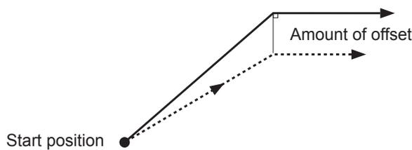
The following explanation describes the tool path when tool-diameter offset is started.
