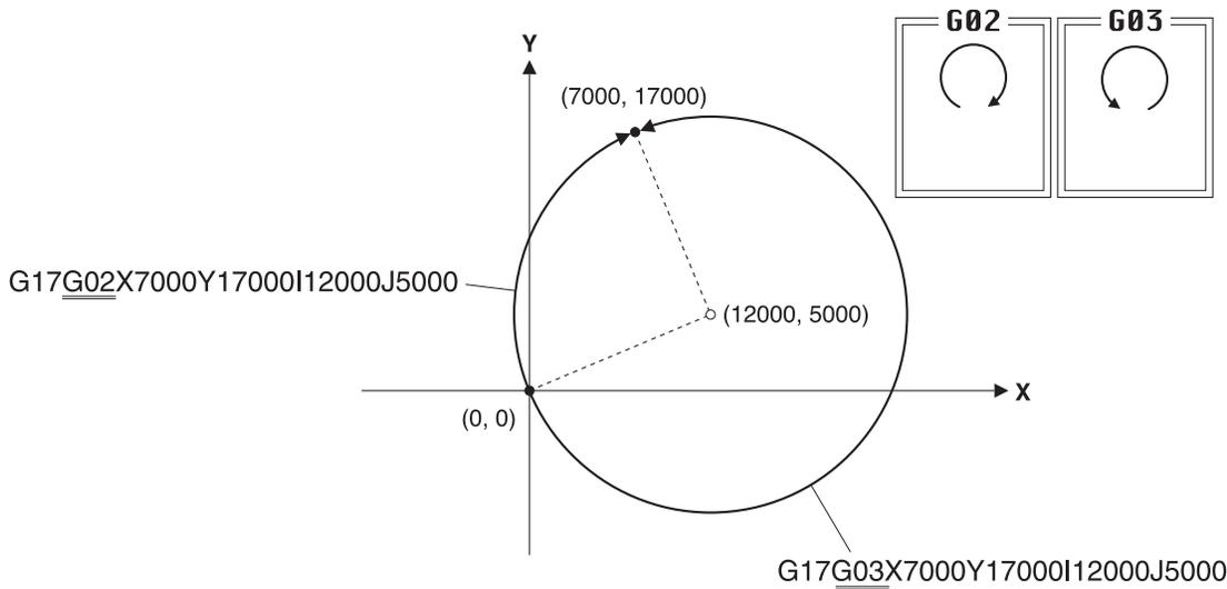
Specifying the radius of the arc (or circle) instead of the arc's center coordinates is also possible. The radius of the arc is specified with R radius. This method is useful when numerical values read from a drawing can be used directly.
