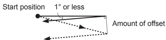
**Operation at Crossover Points During Tool-diameter Offset**
