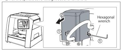
6 Remove the screws using a hexagonal wrench (2.5 mm).
