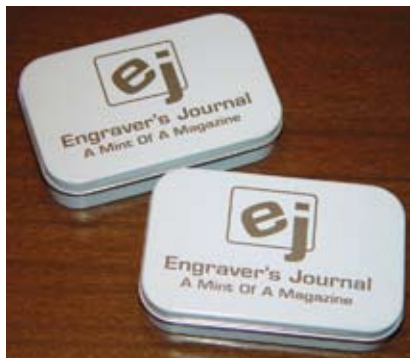
Coated products such as these sublimatable tin boxes marked beautifully with the YAG.
