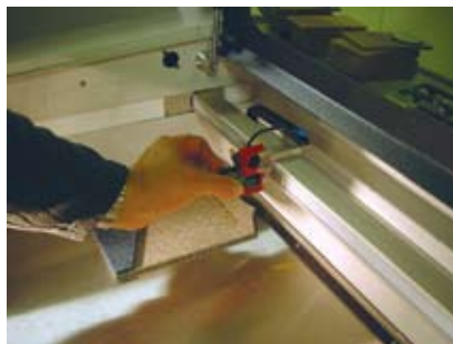
Keeping a clean lens is far more important with a YAG than a CO 2 , so be forewarned; you will have to clean your lens often.
