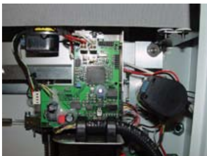
A peek inside the left side of the Hybrid uncovers the electronics for moving the optics from side to side and left to right.
