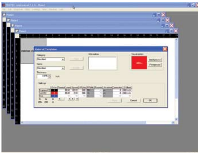
This screen offers you the option of setting power, speed and ppi manually.
