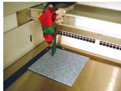
To focus the Hybrid just hang the focus tool in the ledge of the lens assembly and raise the engraving table until the tool falls off.
