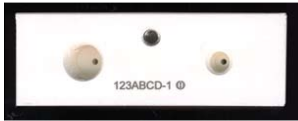
This 1" x 2 3 / 4 " polypropylene block was engraved with a YAG. Notice the engraving turned the plastic black.
