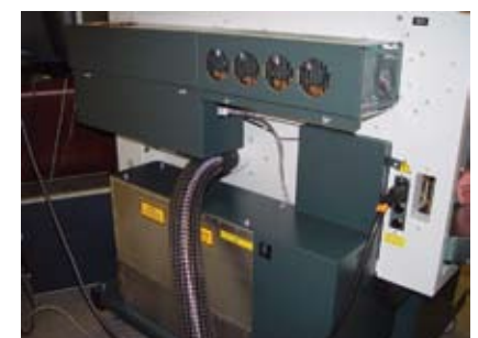
The back of the system is clean and uncluttered and includes the cooling fans, exhaust and electronic connections.
