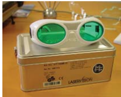
Special safety glasses are required when servicing YAG lasers.
