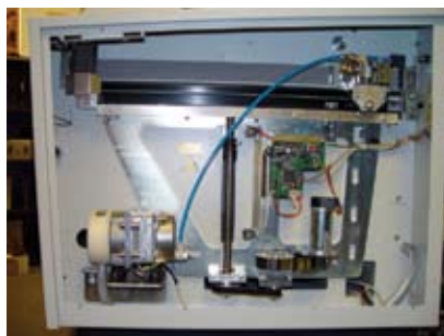
The right side of the machine showcases the motor (lower right) that handles the auto focus and table height adjustments and the motor (lower left) is for the air assist pump.
